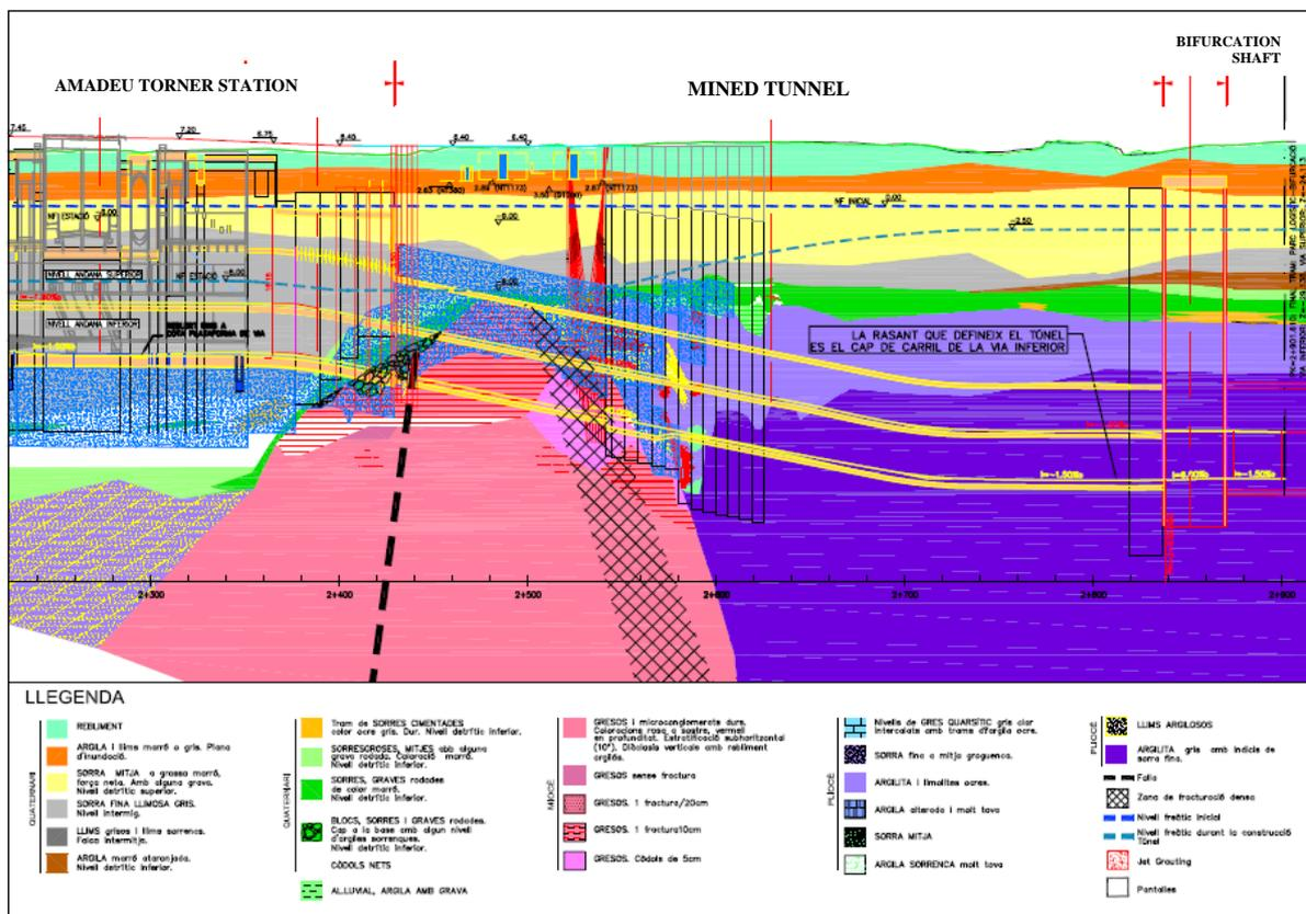
Figure 1 – Geotechnical profile of the stretch built between the Bifurcation Shaft and Amadeu Torner Station
