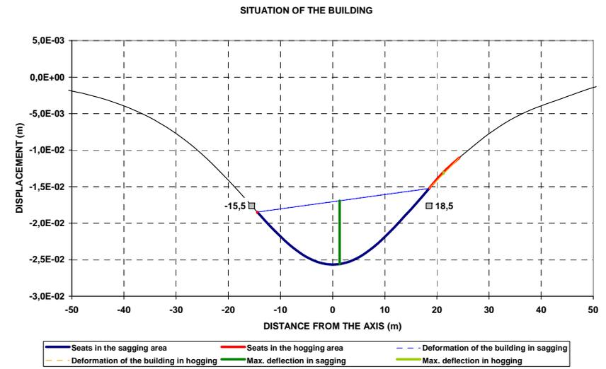
Figure 7 – Calculus of the damages induced to a building
