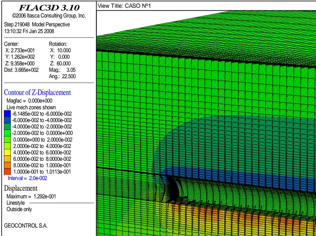
Figure 4 – Distribution of the displacements once the Phase 1 of the excavation has been done
