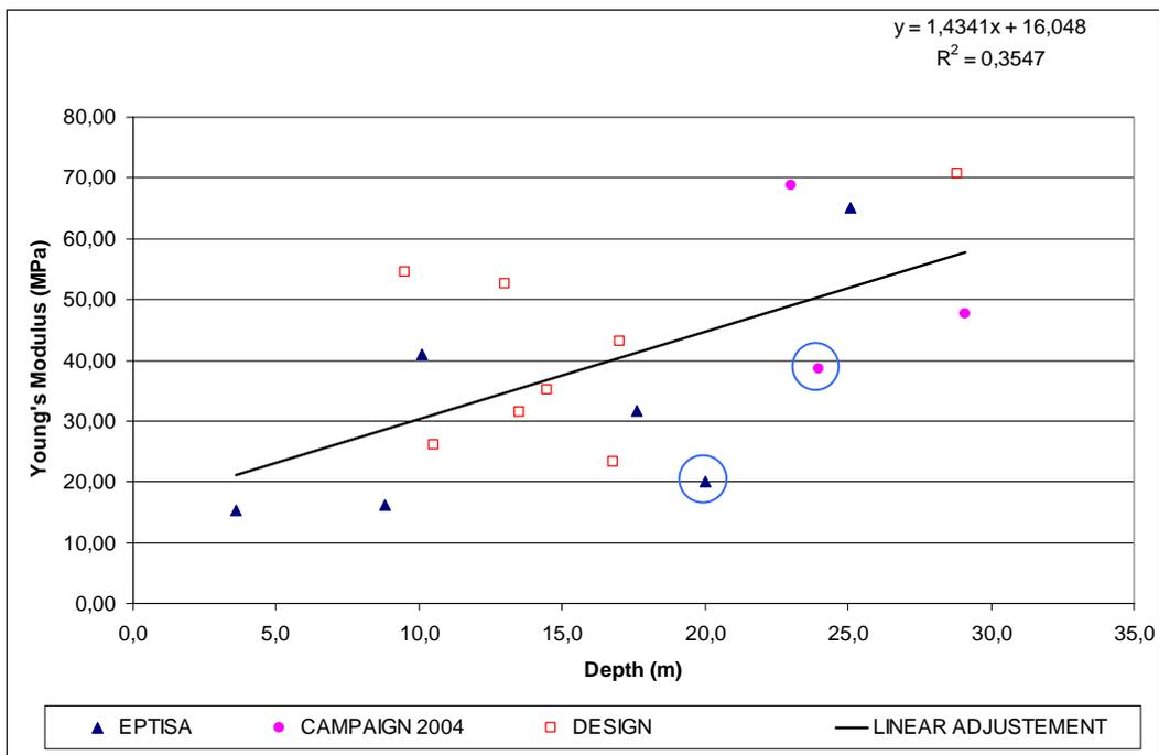
Figure 5 – Adjustment of the modulus of deformation of the soil PL1 with the depth
