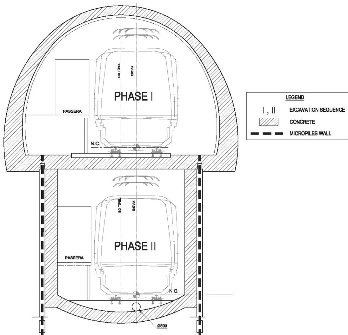
Figure 2- Conceptual design of the tunnel
