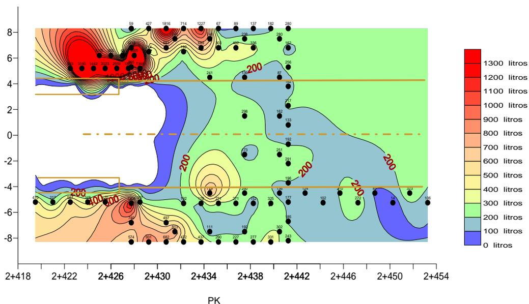
*Figure 8 – Example of the isometric lines of grouted cement intake*
