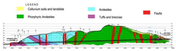
Figure 3. – Geological Cross Section of the Tunnel
