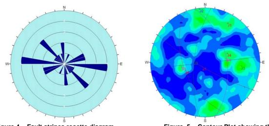
Figure 4. - Fault stripes rosette diagram.
