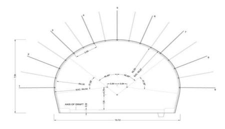
Figure 6. - Excavation Class IV
