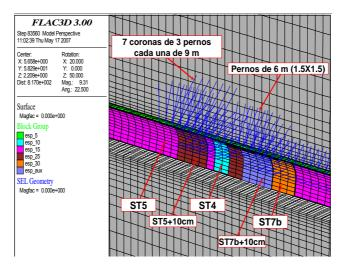
Figure.13. – Detail of the 3D numerical model used for back analysis.
