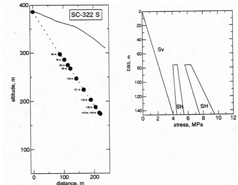
Figure 4 : Natural stress field profiles for borehole SC-322 S (Granodiorites of Le Perthus).
