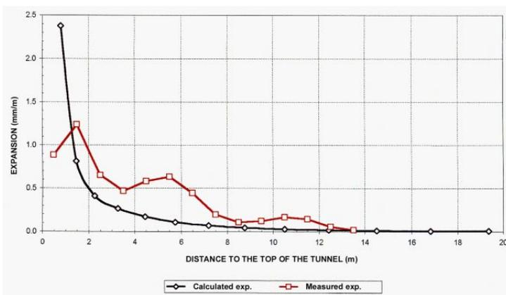
Figure 8 : Correlation between the measured and the calculated expansion at extensometer EV 1.
