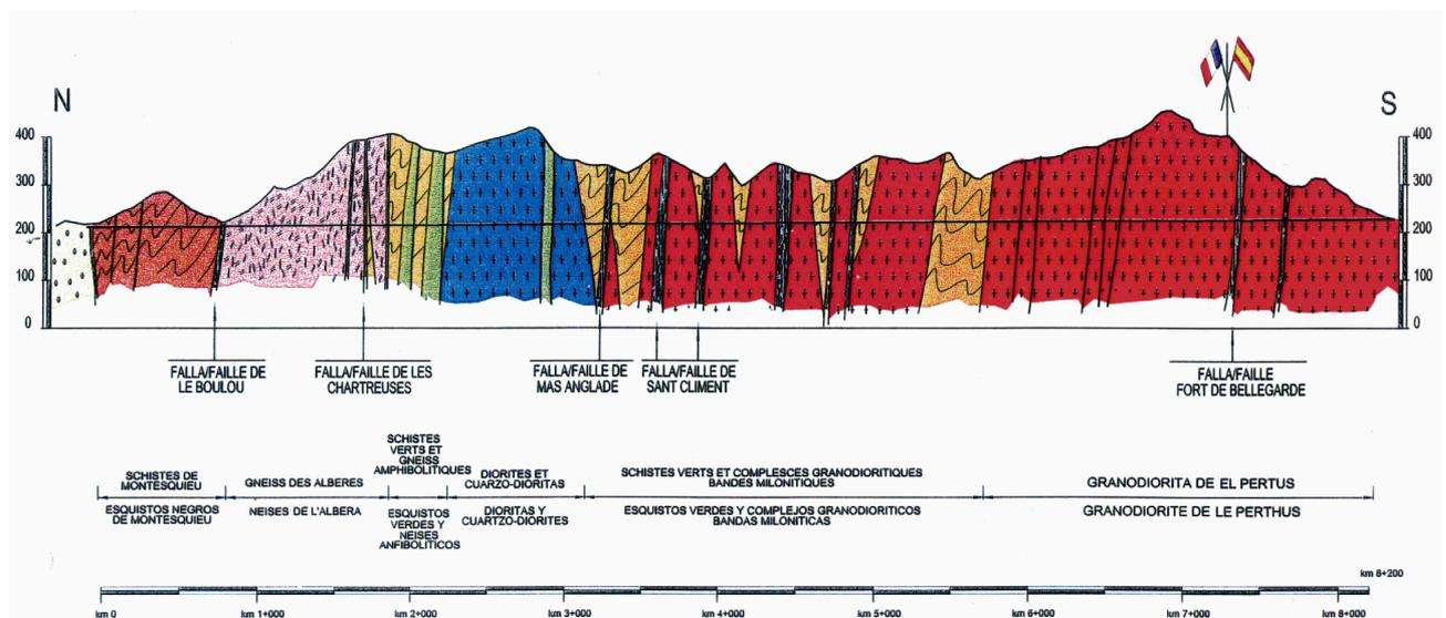
Figure 2 : Geological profile of Le Perthus Tunnel.
