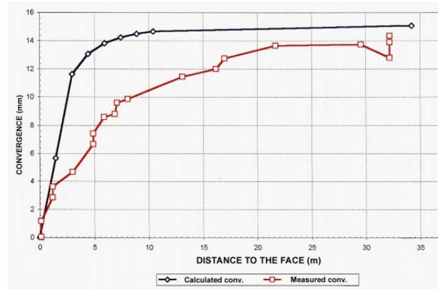
Figure 7 : Correlation between the measured and the calculated convergence.
