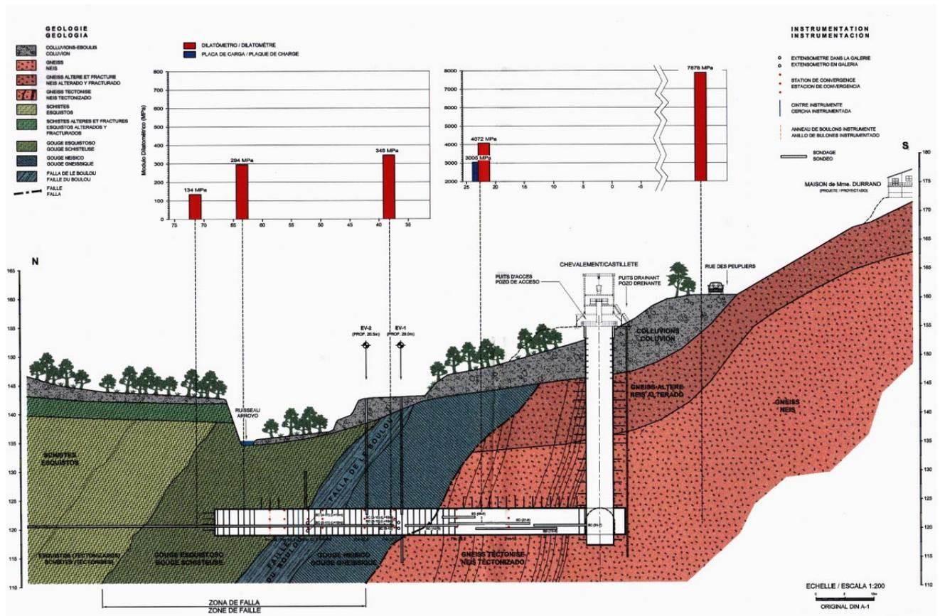
Figure 5 : Geotechnical profile of Le Boulou Experimental Gallery.
