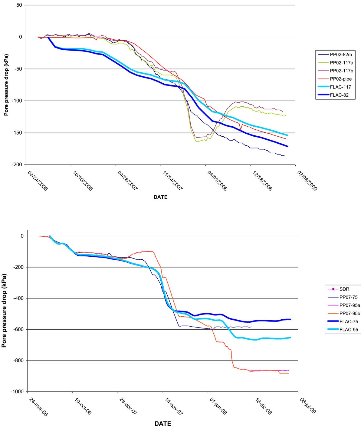
**Figure 8a and 8b** - Evolution of the vibrating wire piezometer sensors PP02 and PP07 compared to FLAC calculation
