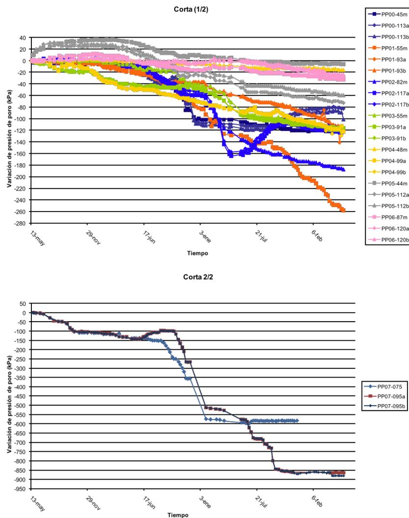
**Figure 4a and 4b** - Evolution of the vibrating wire piezometer sensors
