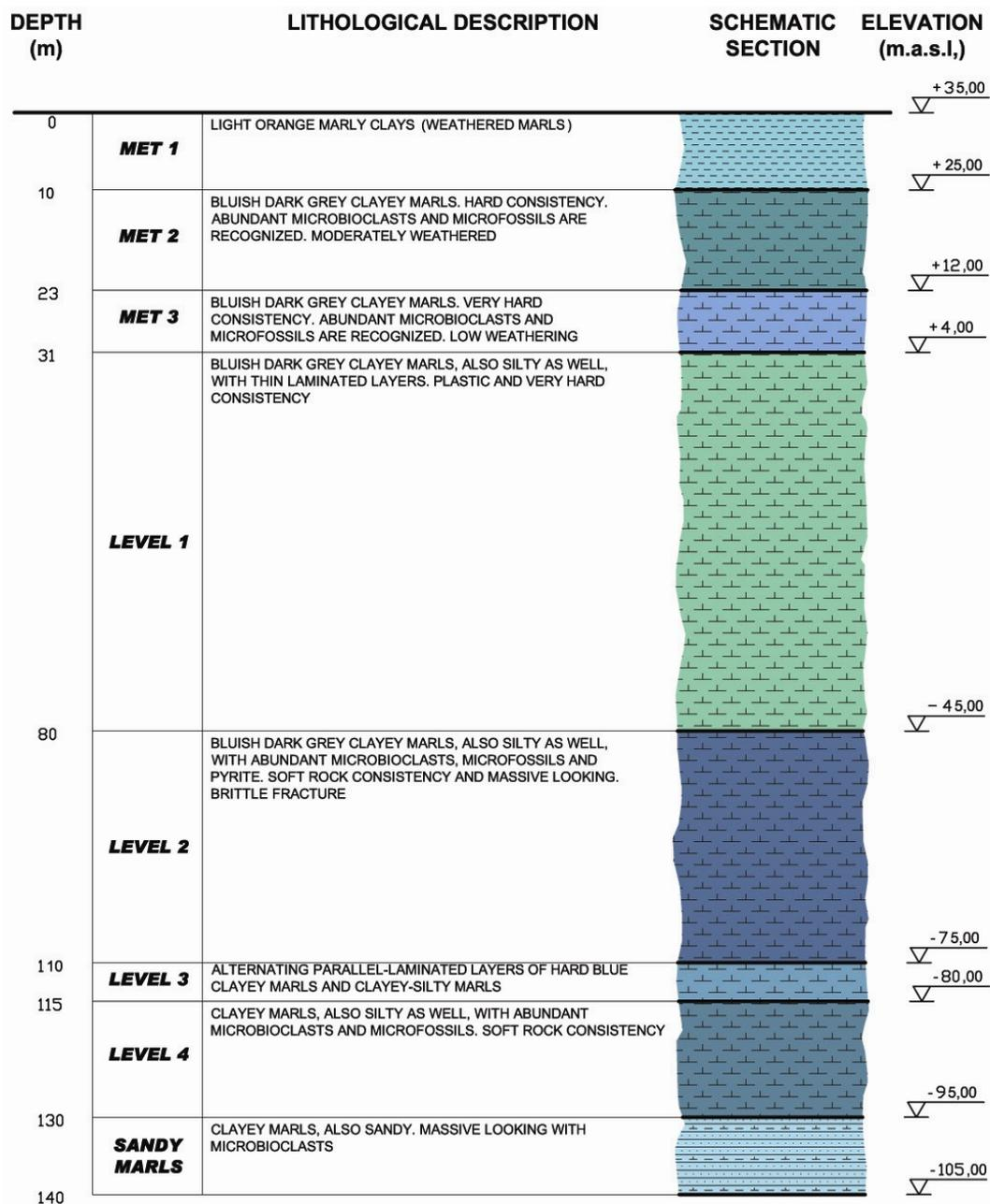
Figure 2 - Lithological Schematic Section
