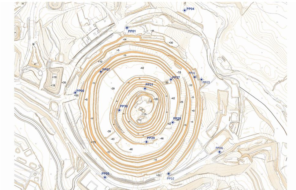
**Figure 3** - Piezometer monitoring net at the pit
