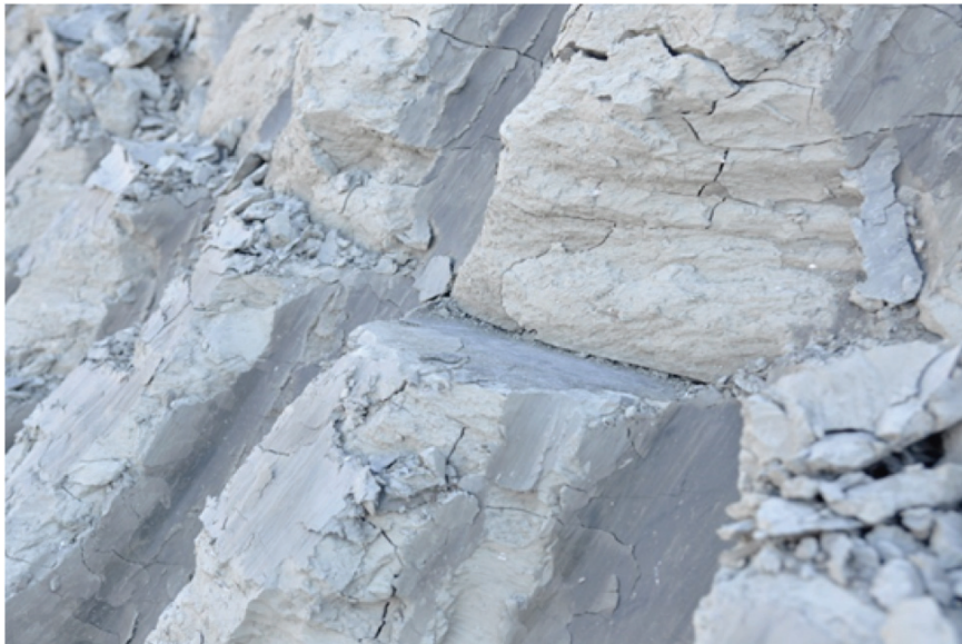
Figure 17 – Displacement observed in bedding plane
