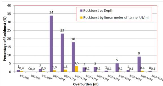
Figure 7: Overburden vs. rockburst and event by meter.
