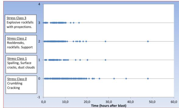
Figure 9: Rockburst intensity vs. time after blasting
