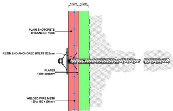
Figure 12: Rocksupport designed for high stress levels.
