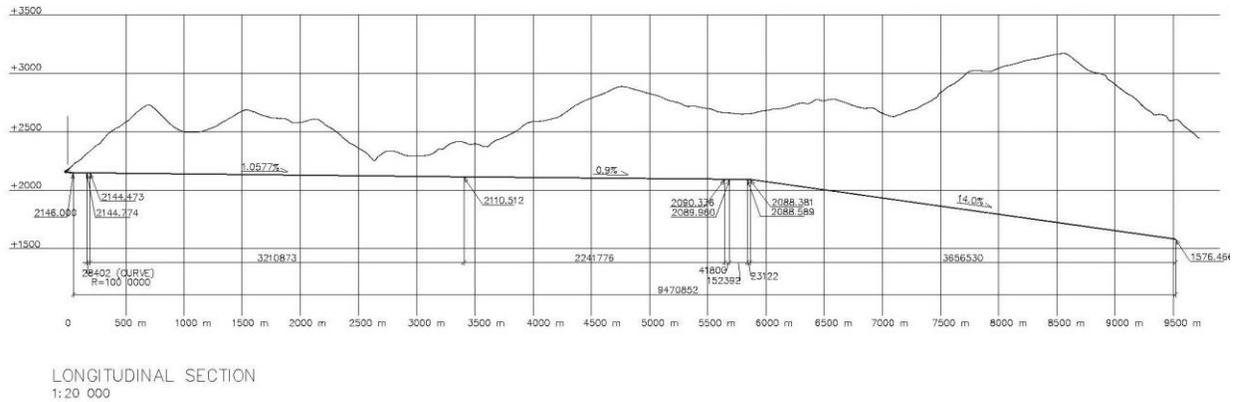
Figure 1: Longitudinal section of Cheves Hydropower project
