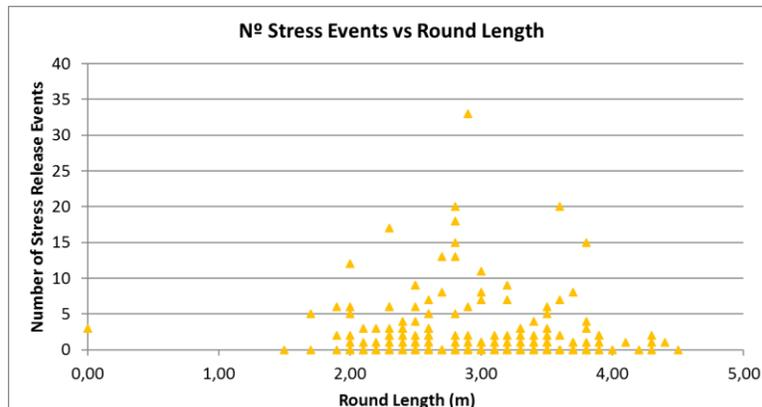
Figure 10: Blasting length vs. number of events
