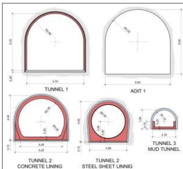
Figure 4. Sections of the main underground structures.
