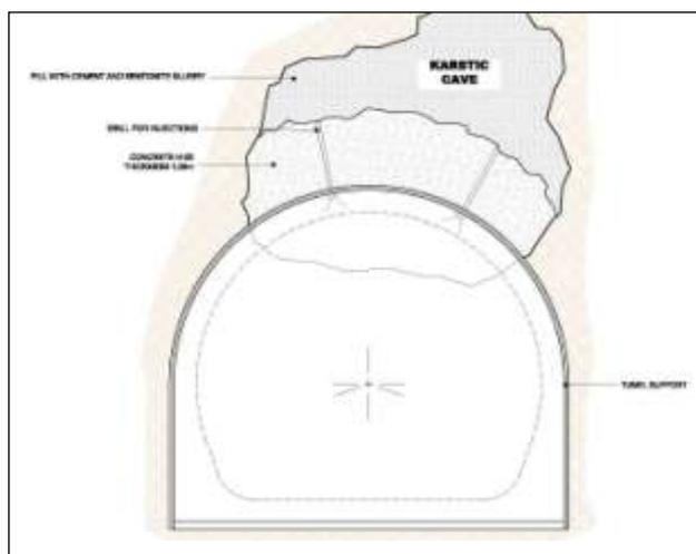
Figure 5. Section for caves intersection at the roof/walls.
