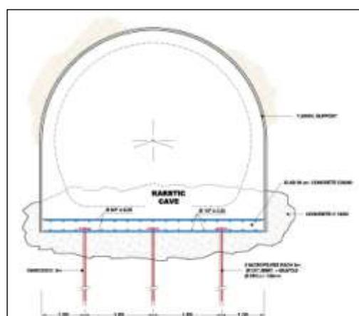
Figure 6. Section for caves intersection at the floor.
