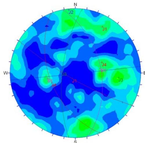
**Figure 5. - Contour Plot showing the five joint sets detected**
