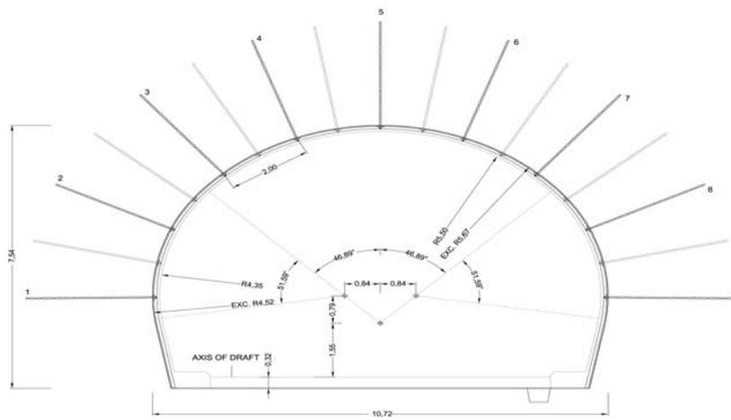
**Figure 6. - Excavation Class IV**
