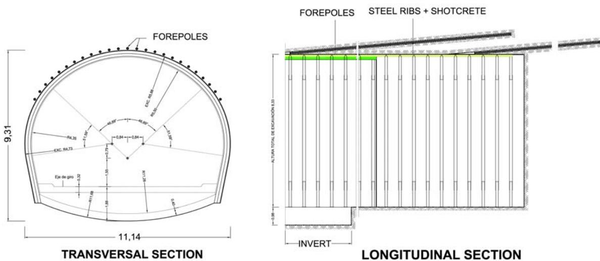
**Figure 7. - Excavation Class VII**
