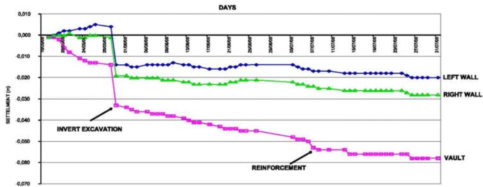
Figure 9. - Descent of the tunnel vault in the convergence station measurement C2 PK 2+720
