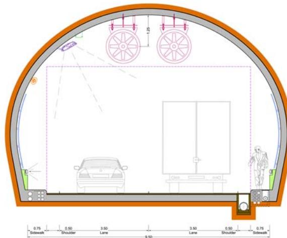
Figure 1. – Tunnel Section
