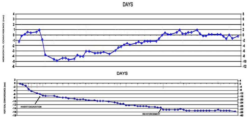
Figure 8. – Convergence Station measurement C2 PK 2+720
