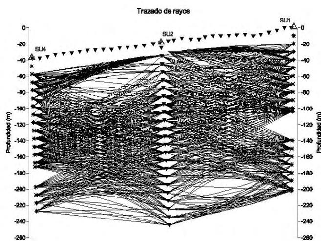
Figura 7.- The raypaths of one of the sections measured with seismic tomography in La Umbria Fault zone.
