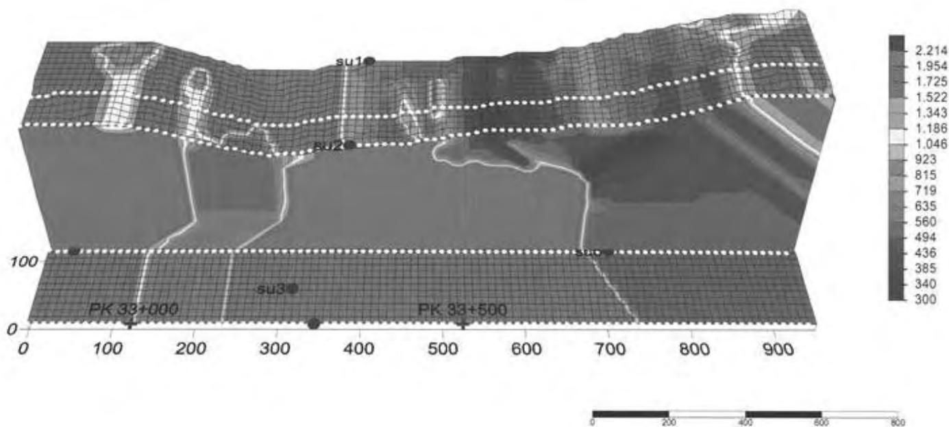
Figura 6.- Resistivity 3D model of La Umbria Fault zone. (In the horizontal plane, both tunnel axis have been marked).
