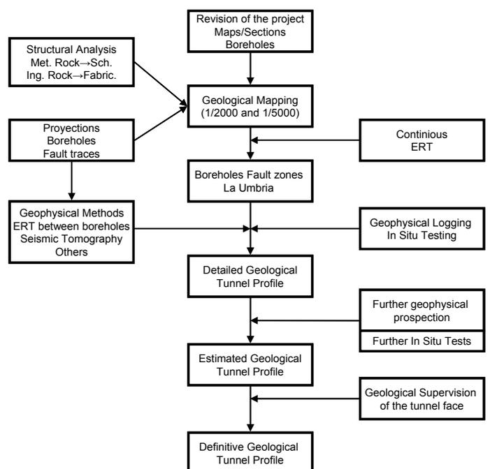
Figure 3.- Methodology used for the prediction of the ground conditions ahead the TBM face (modified from Capote, 2005).
