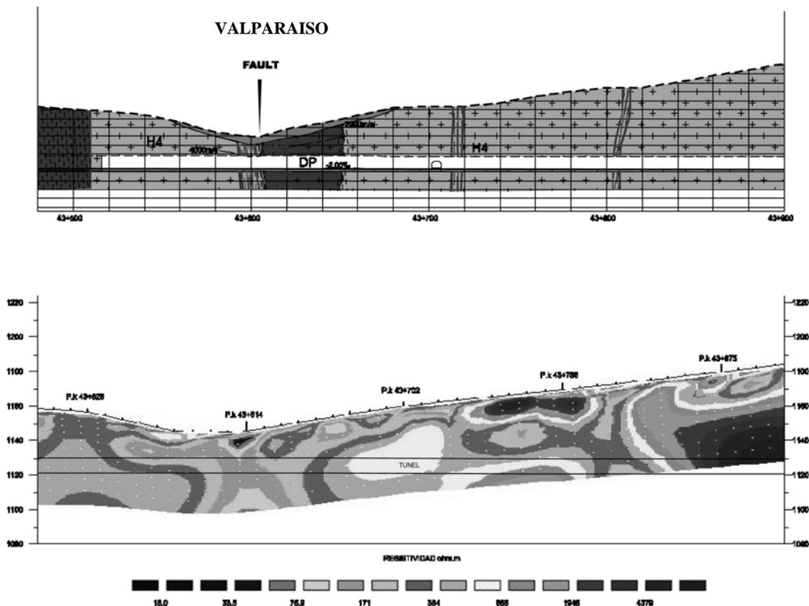
Figure 5.- Example of the correlation between the resistivity and the geological profiles. (Valparaiso Fault).
