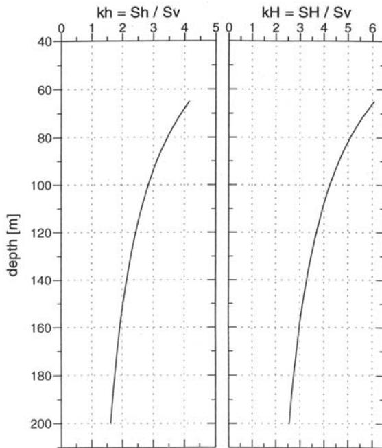
Figura 9.- Result of the Hydrofract tests carried out in one borehole, showing high horizontal stresses.
